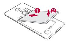
4 To replace the cover onto the device, align the back cover over the battery compartment and press it down until it clicks into place.
