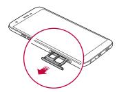
3 Put the SIM card on the card tray with the gold-coloured contacts facing downwards.
